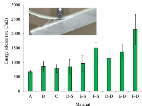
Figure 4: Summary of the interfacial fracture properties of the sandwich structures
