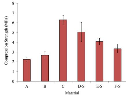
Figure 3: Summary of the compression strength of the core materials
