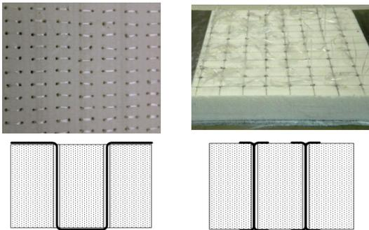
Figure 1: Schematic and pictures of the patterns for the through-thickness fiber reinforcement in the PET foam.
