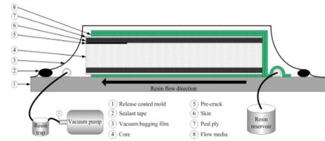
Figure 2: Schematic of the VARTM process
